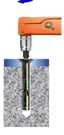
Tighten to recommended torque
